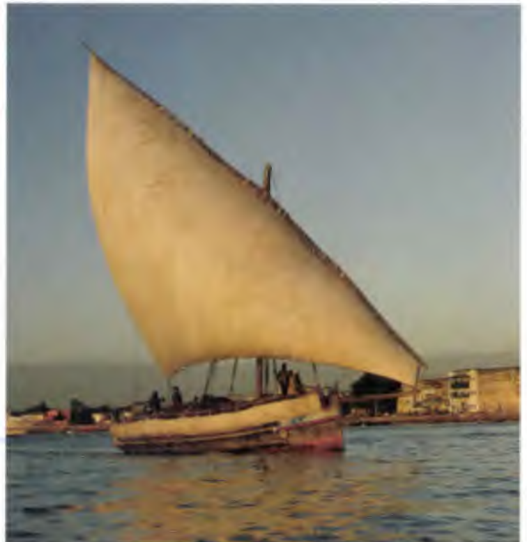
FIGURE 8-36 The dhow is a traditional Arabian vessel with a triangular sail. The largest ocean-going dhows had two masts. Arab traders sailed dhows in Middle Eastern waters, and to Africa, India, and China.
