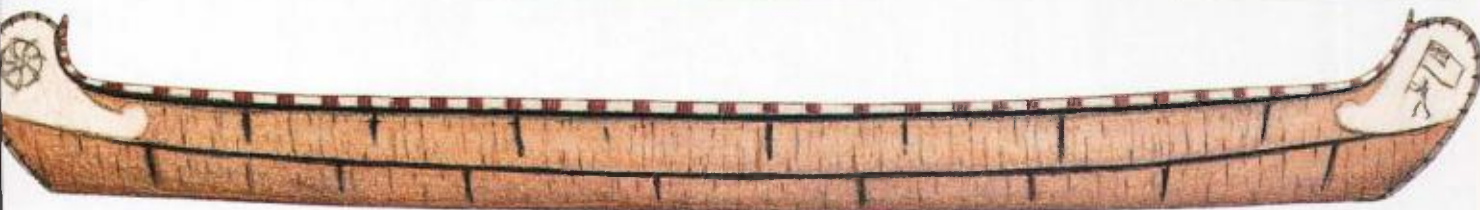
Figure 9-15 The canoes used to transport goods from Montreal to Fort William were called canots de maître . They were about 10 or 11 metres long and about one and a half metres wide, used twelve paddlers, and could carry 4 tons [4000 kilograms] of weight.
