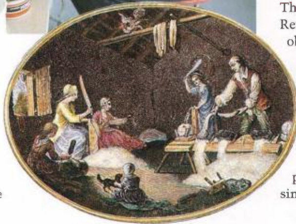
Figure 5-13 An engraving of cottage industry, 1783. These people are preparing flax for the manufacture of linen in a cottage in County Down, Ireland. Likely they are all family members, but we do not know because they have not been identified.
