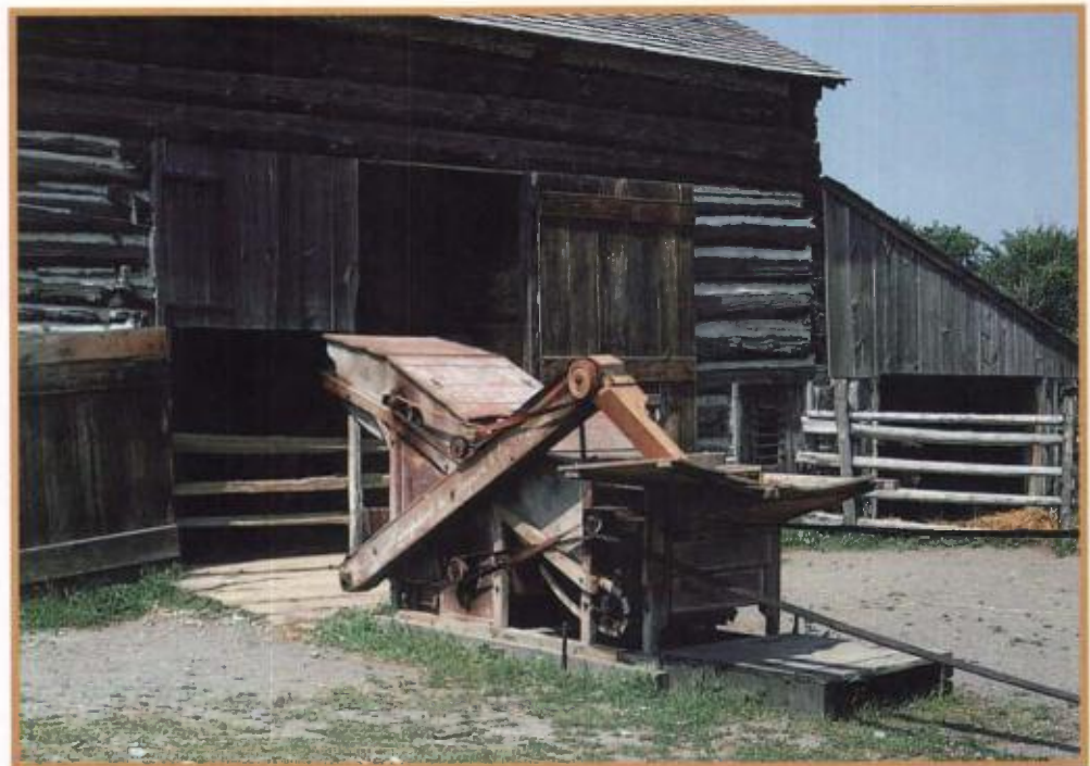
Figure 10-19 Loyalists and other settlers were forced to clear land and build houses and barns before their farms could be profitable. Their three basic products, wheat, lumber, and potash , helped provide money for survival and improvements. Opposite, a thresher stands outside a recreated pioneer farm house in Ontario.
