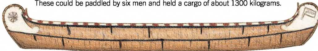
FIGURE 3-18 The small canoes used from the interior to Fort William were called canots du nord. They were 7 metres long and a little over a metre wide. They had to be small because the route mainly followed rugged rivers with multiple portages. These could be paddled by six men and held a cargo of about 1300 kilograms.
