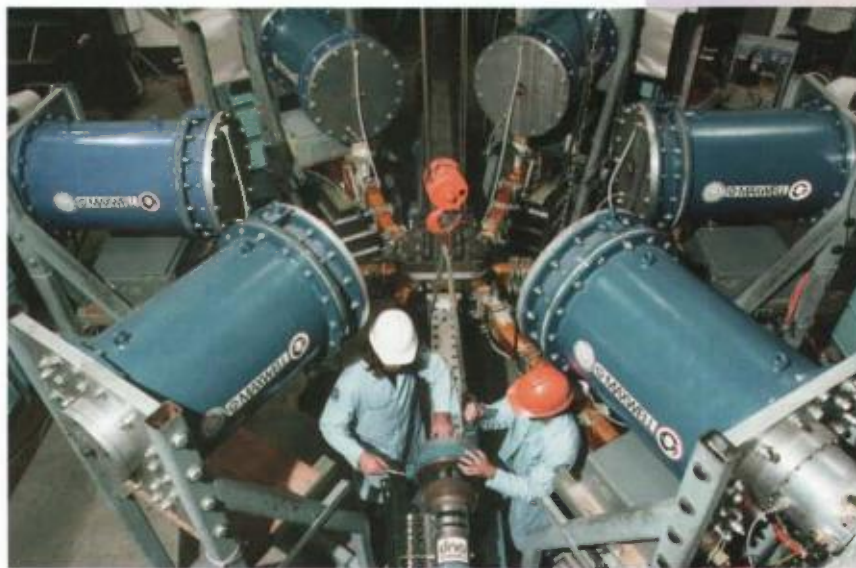
Figure 18-8 Technicians working on the U.S. Strategic Defence Initiative ("Star Wars") align a rail gun—a device that uses electromagnetism to accelerate particles to very high speeds—towards a target.
