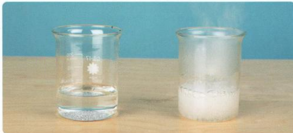
Figure 3 The beaker on the right has a higher concentration of hydrochloric acid reacting with zinc metal, which results in a higher rate of reaction than the beaker on the left.
