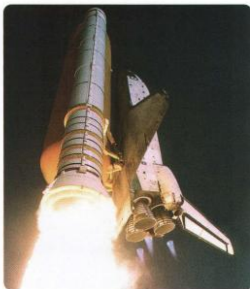
Figure 4 The three shuttle engines produce colourless water vapour during launch. The three blue cones of light coming from the engines are called blue mach diamonds. Their presence and distance from the main engines indicate a good lift-off.
