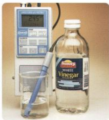
Figure 7 A pH meter can be used to accurately measure the acidity of a solution.
