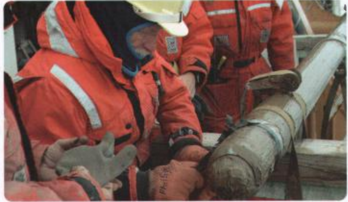
This vertical sediment core is extruded into slices which correspond to discrete time intervals.
