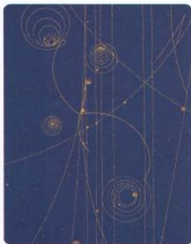
Figure 5 Tracks made by alpha and beta particles in a bubble chamber
