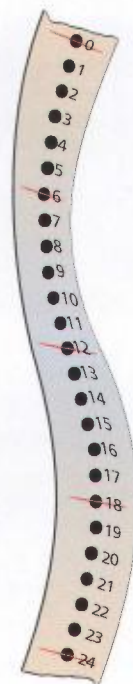
Figure 2 Sometimes it is more convenient to use time intervals of six dots rather than using every dot.
