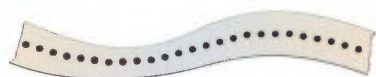
Figure 2 The spacing of the dots on the tickertape indicates the rate of motion.
