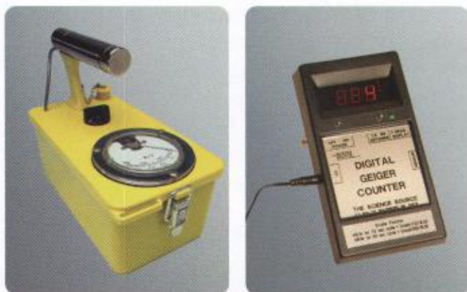
Figure 1 Geiger counters are particle detectors that measure ionizing radiation. There are several different types of Geiger counters that you may see in your studies.
