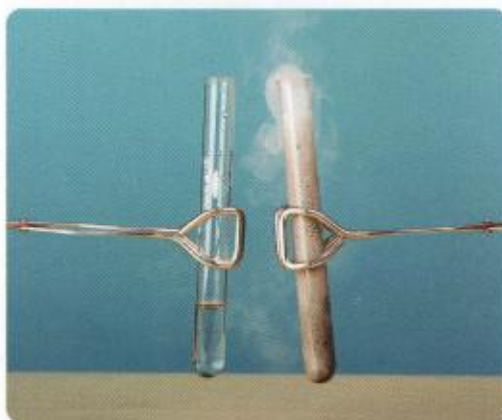
Figure 4 Water and hydrogen peroxide have different ratios of hydrogen atoms to oxygen atoms, and are therefore, different compounds. This is seen in their different properties, as the hydrogen peroxide in the right tube is reacting in the presence of the solid compound \text{MnO}_2 , and the water in the left tube is not.
