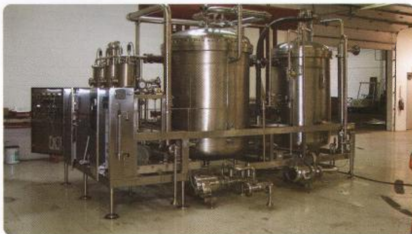
Figure 1 Your favourite soft drink is produced in a carbonation system like this. The machine mixes water with a flavoured syrup and then infuses it with carbon dioxide before cooling.
