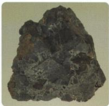
Figure 1 Pitchblende, the major uranium ore, is a heavy mineral that contains uranium oxides, lead, and trace amounts of other radioactive elements. Pierre and Marie Curie found radium and polonium in pitchblende residues.
