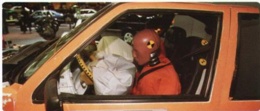
Figure 2 Deflation of an airbag begins immediately after deployment to protect the person from injury caused by the sudden inflation.
