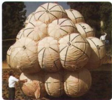
Figure 1 The Mars Pathfinder's airbags were tested under simulated Martian conditions.
