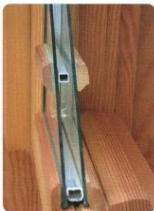
Figure 5 Windows like this one are made to reduce heat loss in three ways. The special glass is a poor transmitter of radiation; the layer of trapped gas between the panes is very thin, reducing convection; and the noble gas used to fill the space is a poor conductor.
