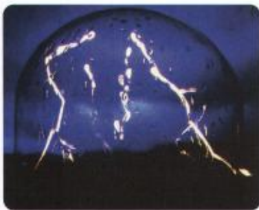
Figure 4 In a cloud chamber, the alpha particles produce a thick, short track. Beta particles make a thin irregular track. Gamma rays have no charge and, thus, no track.
