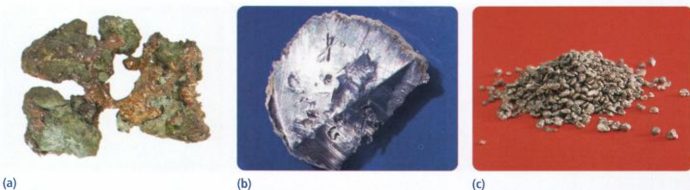
Figure 5 Samples of elements: (a) copper, Cu; (b) potassium, K; (c) calcium, Ca.
