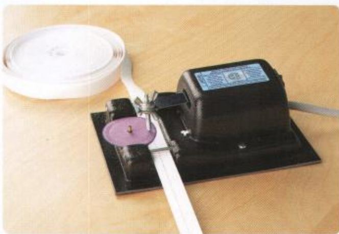
Figure 1 A recording timer can be used to time motion.
