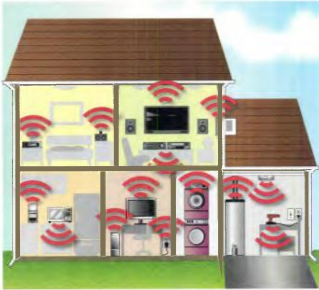
Figure 3.32 Devices with phantom loads are common in a typical home. Identify the devices with phantom loads in this figure. For each device, explain why you think it has a phantom load.
