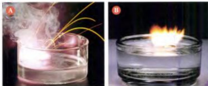
Figure 2.21 Potassium A is more reactive than sodium B because less energy is needed to remove the valence electron from potassium.
