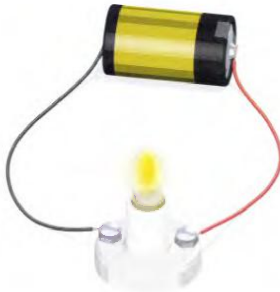
Figure 3.19 A closed loop allows current to flow and light the bulb. Short circuits can be dangerous if they occur in the wiring of a building. Suggest how a short circuit might form in a building.
