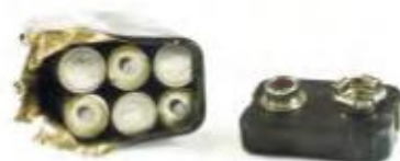
Figure 3.14 The battery shown here is made up of six individual cells.
