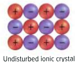
Figure 2.25 When a force strong enough to overcome the strong forces of attraction between oppositely charged ions is applied, ions with like charges come close together. They repel one another and the solid cracks.
