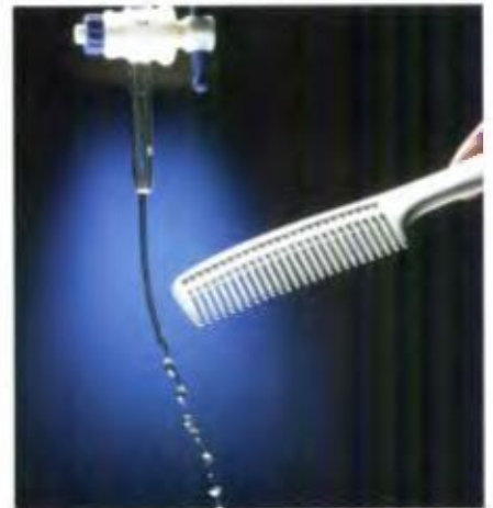
Figure 3.11 In this photo, the comb is charged, and the water is neutral.
