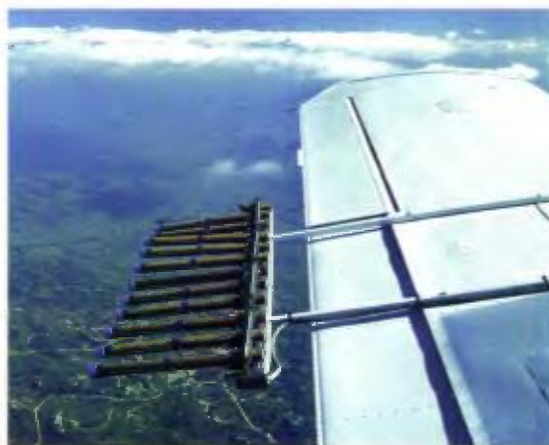
Figure 2.40 Silver iodide generators are designed for cloud seeding.
