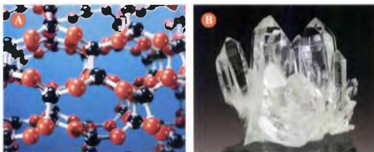
Figure 2.34 A Silicon dioxide, quartz, is a network solid. Its atoms are bonded into a regular, repeating structure by covalent bonds. This model shows a small part of the structure. In real quartz crystals like the ones shown in B , billions of atoms are bonded together in this same repeating structure, forming one giant molecule.
