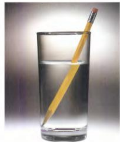
Figure 3.22 This pencil appears broken due to refraction. In reality, the bottom part of the pencil is not where your brain thinks it is.
