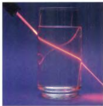
Figure 3.21 This beam of red light allows you to see the path of light bend as it enters and leaves the water.
